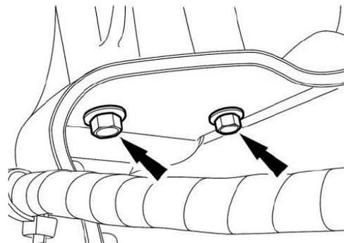
14. Position back the oil level indicator and tube and install the nut.
