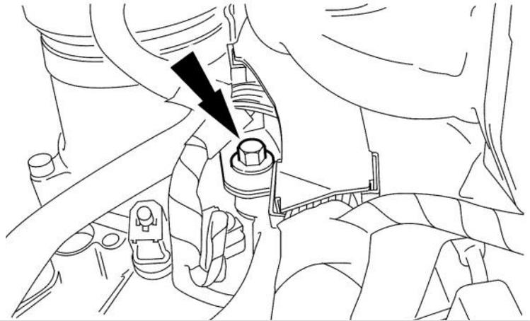
34. Use a commercially available disconnect tool and a screwdriver to release the fuel tube.
