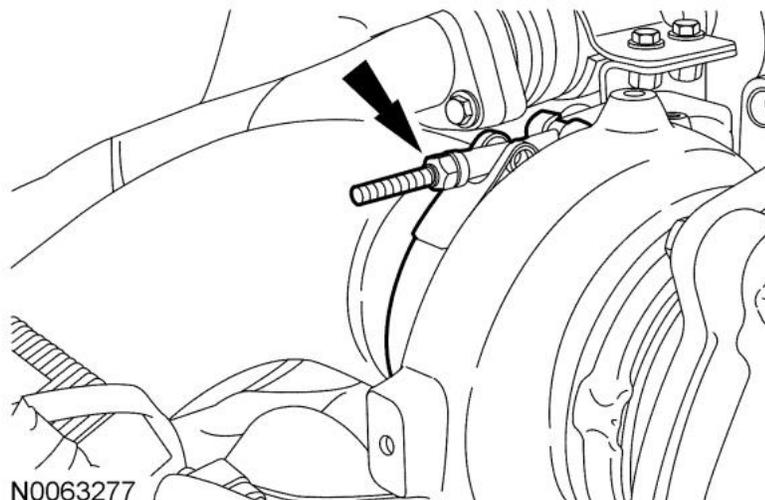
25. Remove the 6 turbocharger inlet pipe bolts and EGR-OC-to-turbocharger bracket.
