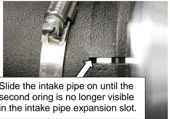
Slide the intake pipe on until the second oring is no longer visible in the intake pipe expansion slot.
