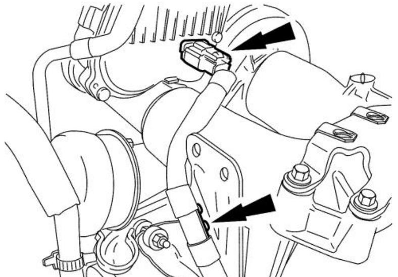
14. Remove the 2 RH turbocharger inlet pipe-to-EGR-oxidation Catalytic converter (OC) pipe bolts and the 2 EGR-OC-to-turbocharger
