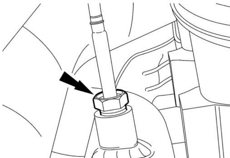
**NOTE:** Index-mark the drive shaft prior to disconnecting from the axle.
