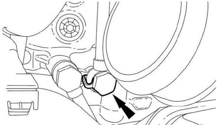
16. Install the fuel filter element and cover.
