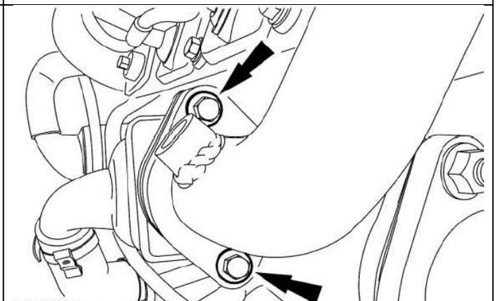
29. Tighten the 2 EOR-OC pipe bolts at the RH turbocharger inlet pipe.
