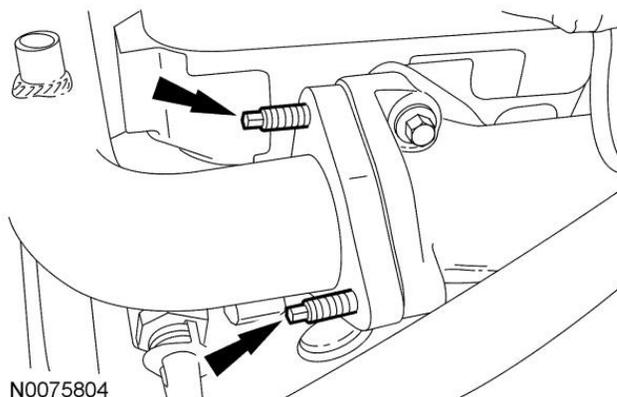
28. Loosen the clamps and remove the Charge Air Cooler (CAC) tube flex coupling.
