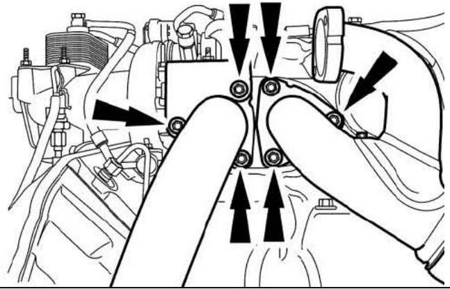
**21. NOTICE:** Due to limited access, one of the specific Half-moon wrenches and other tools described must be used to correctly tighten the fasteners in this step. Failure to follow this instruction may result in engine failure.
