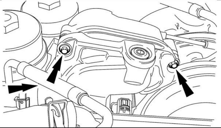
12. Remove the fuel cooler bracket.
