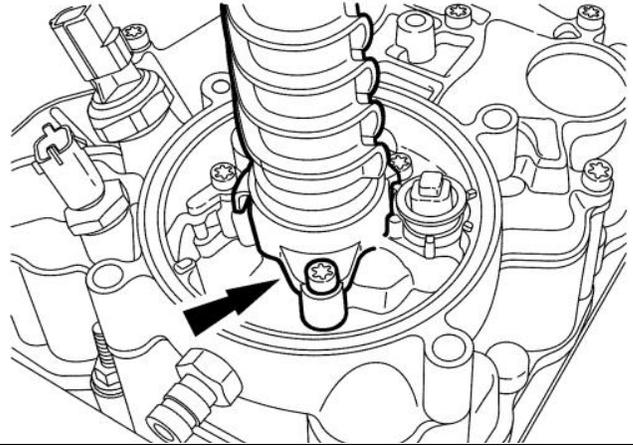
38. Remove and discard the oil filter base gasket and seal.
