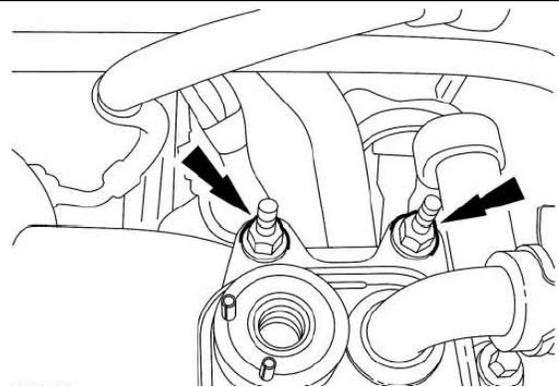
43. Install the 2 bolts for the fuel cooler.
