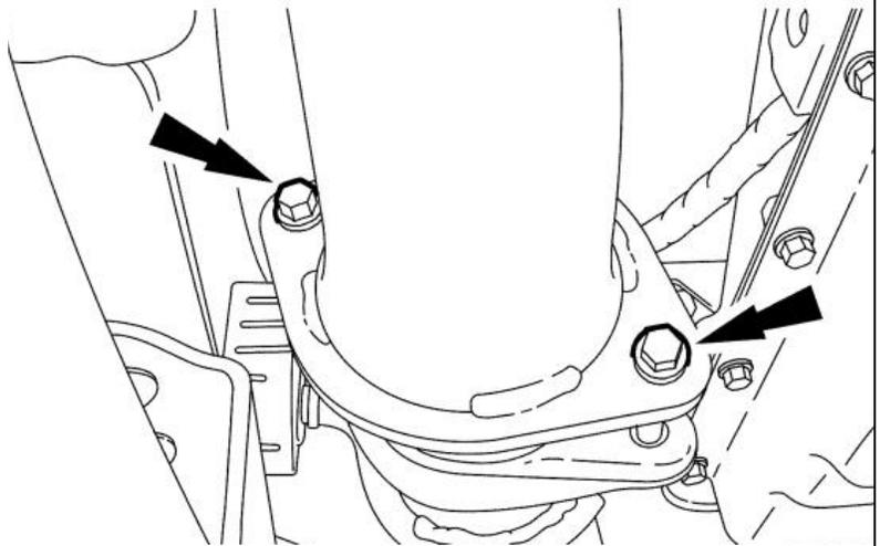
23. *NOTE:* LH Shown, RH Similar. Remove and discard the 6LH and RH turbocharger inlet pipes-to-exhaust manifold nuts.
