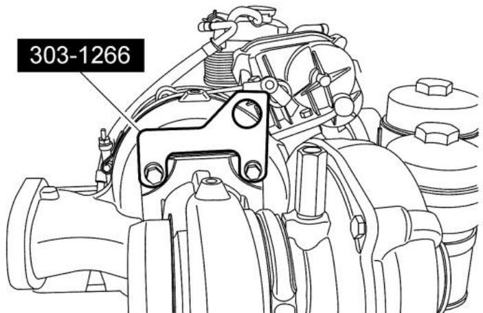
**NOTICE:** Failure to use the turbocharger lifting bracket during removal, handling or installation of the turbocharger could result in a low pressure to high pressure turbocharger seal failure.
