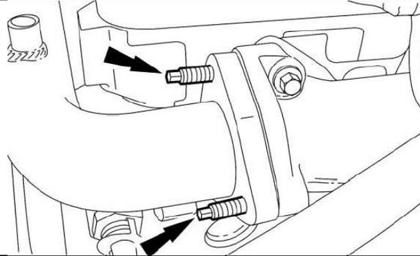
19. **NOTICE:** Do not bend or twist the turbocharger inlet pipe or damage to the turbocharger inlet pipe may occur.
