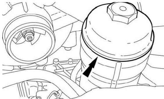
11. Connect the fuel injection pump supply tube at the fuel filter module.
