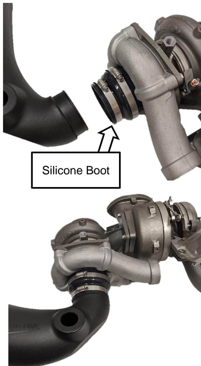
**1047080/81 ONLY** - Do not use reducer bushing from kit. Disregard step 9 from the AFE intake manual.
