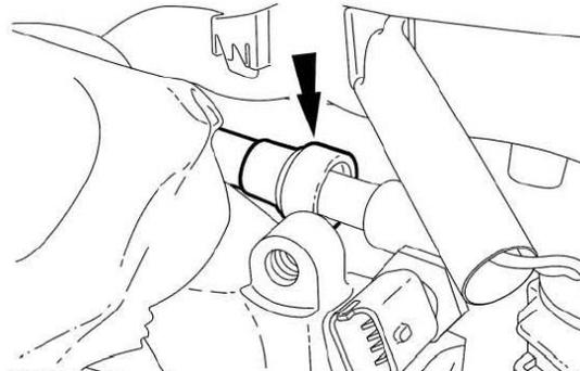
12. Install the bolt for the engine wiring harness.
