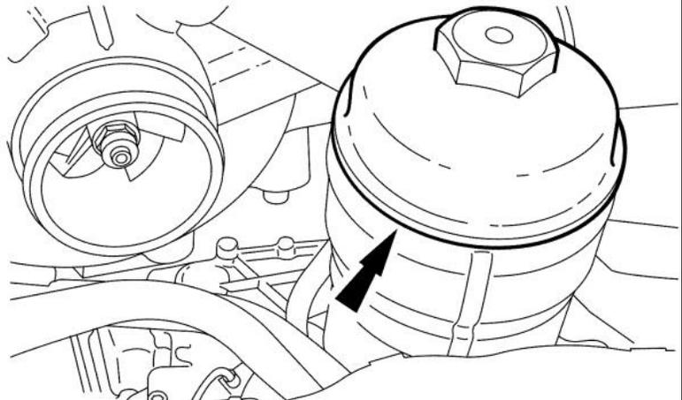
36. Remove the 4 torx bolts and the oil filter housing.
