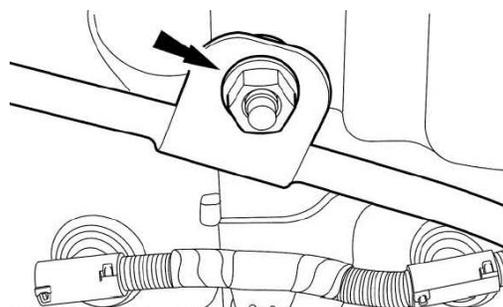
15. **NOTICE:** Use only banjo bolts with a green hex head. The green-headed bolts do not contain a check valve. When viewed from the inner end, the correct bolt will appear open. Failure to install the correct banjo bolt may result in damage to the fuel system.
