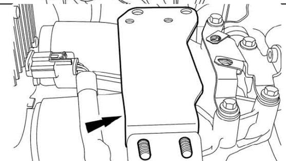
40. Position back the fuel cooler, fuel cooling system expansion tank and turbocharger actuator cooler. Install the 3 bolts for the turbocharger actuator cooler. Tighten the bolts in the sequence shown in 2 stages.
