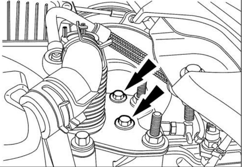
9. Remove the 2 stud bolts for the fuel cooler.
