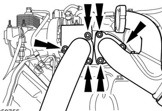
26. Remove the 3 LH turbocharger inlet pipes-to-exhaust manifold studs and gasket. Remove the LH turbocharger inlet pipe.
