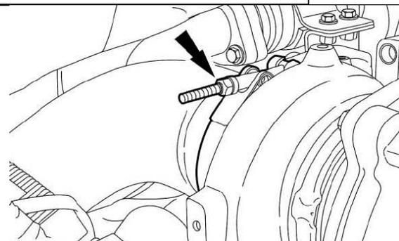
25. **NOTICE:** Make sure the correct bolts are installed in the bracket or damage to the bracket can occur.
