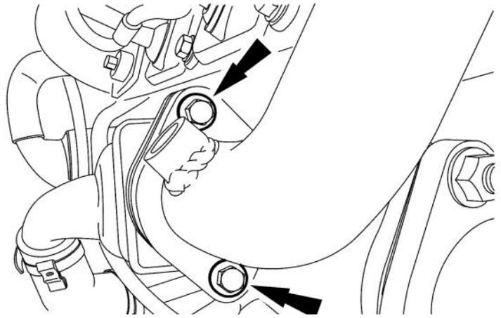
22. Loosen the 2 exhaust downpipe-to-OC pipe bolts.
