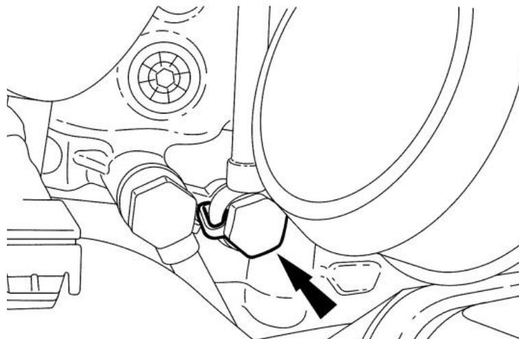
31. Remove the nut and position the oil level indicator and tube aside.
