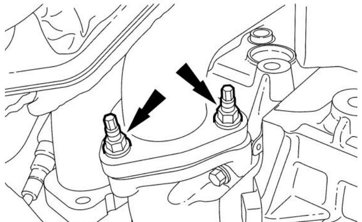
24. Remove and discard the exhaust downpipe clamp. Position aside the exhaust downpipe.
