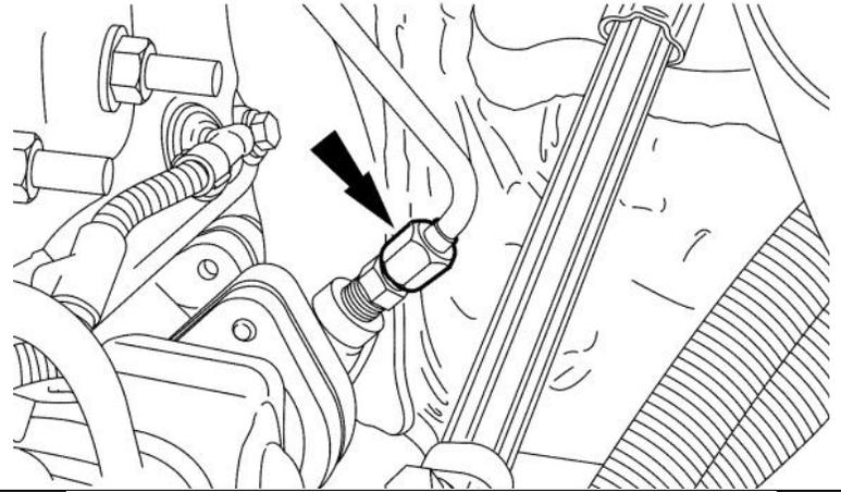
19. Remove the EP sensor tube fitting from the EGR-OC pipe.
