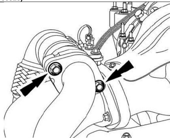
30. Tighten the 2 bolts for the EOR-OC pipe bracket at the turbocharger.
