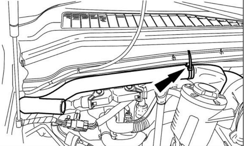
**NOTICE:** Do not lean on, pull on or use the turbocharger oil supply tube as a handle or damage to the turbocharger oil supply tube may occur.
