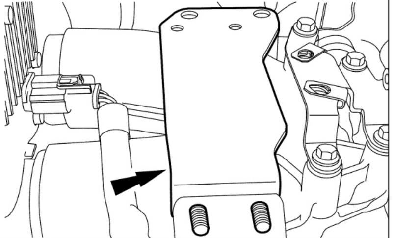
13. Disconnect the turbocharger actuator electrical connector and pin-type retainer.
