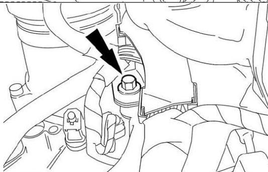
13. **NOTE:** Rear bolts shown, front bolts similar. Position the front fuel cooler bracket. Install the 4 bolts for the turbocharger crossover tube.
