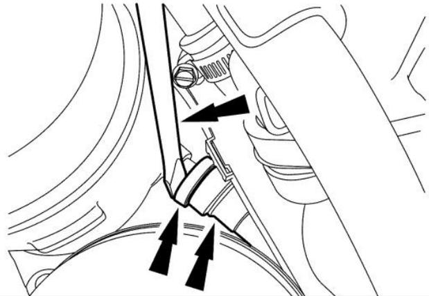
35. Remove and discard the oil filter element and O-ring seal.
