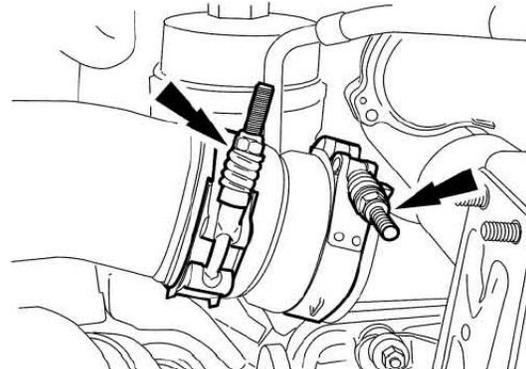
18. Install the 2 new studs for the RH turbocharger inlet pipe.
