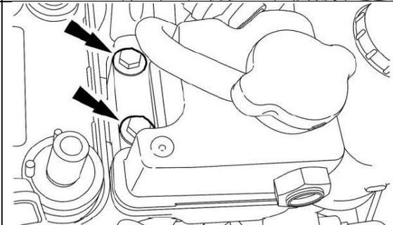
**45. NOTICE:** Use only banjo bolts with a green hex head. The green-headed bolts do not contain a check valve. When viewed from the inner end, the correct bolt will appear open. Failure to install the correct banjo bolt may result in damage to the fuel system.
