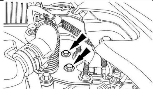
44. Install the 3 bolts for the fuel cooling system expansion tank.
