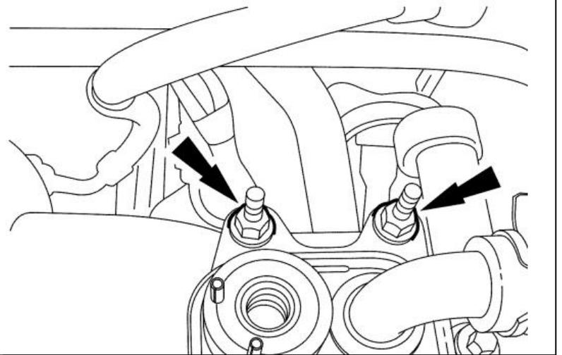
10. Remove the 2 nuts for the fuel cooler.
