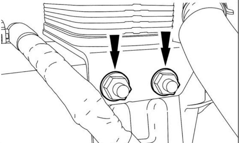
11. Remove the 3 bolts for the turbocharger actuator cooler. Position the fuel cooler, fuel cooling system expansion tank and turbocharger actuator cooler aside.
