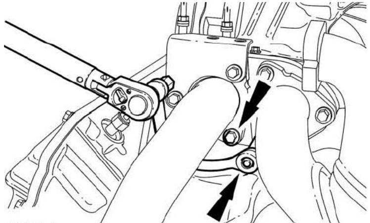
**Torque Chart - Turbocharger Inlet Pipes-to-Turbocharger,
