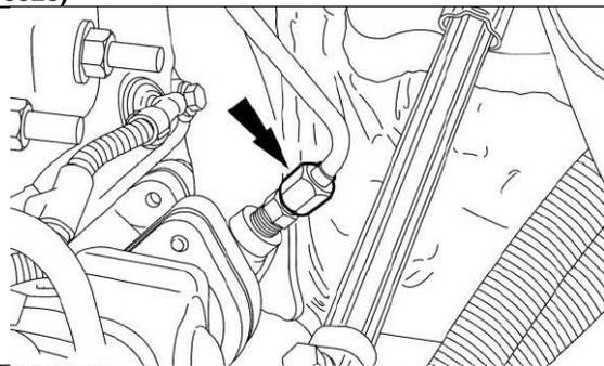
35. If equipped, position back the front driveshaft and install the 2 straps and 4 bolts.
