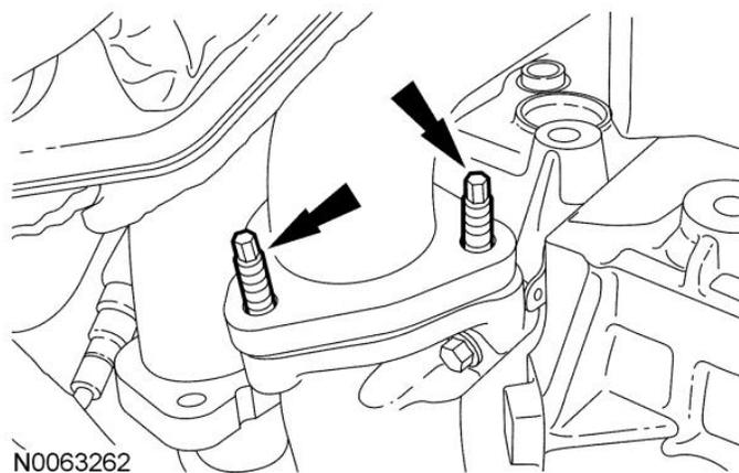
27. Remove the 2 outer RH turbocharger inlet pipes-to-exhaust manifold studs.
