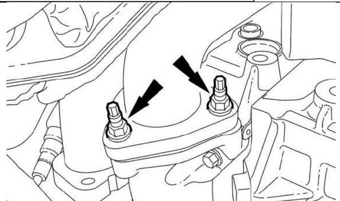
23. **NOTICE:** Due to limited access, one of the specific Half-moon wrenches and other tools described must be used to correctly tighten the fasteners in this step. Failure to follow this instruction may result in engine failure.
