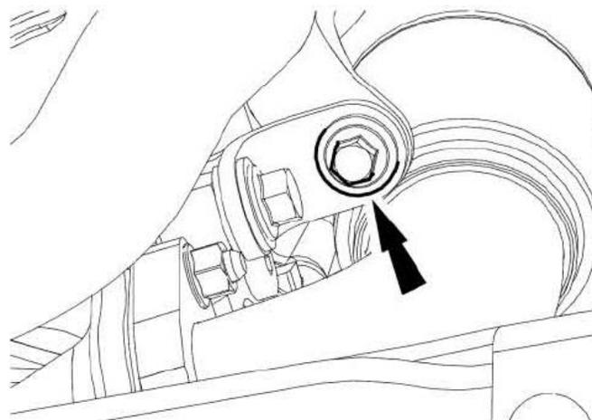
32. **NOTICE:** Failure to install and correctly tighten the Exhaust Gas Recirculation (EGR)-Oxidation Catalytic Converter (OC) pipe support bolt will result in damage to the horizontal EGR cooler and possible engine damage.
