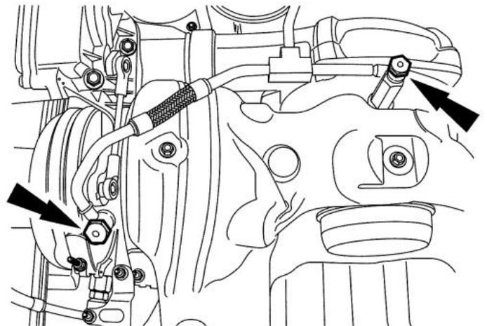
4. Remove the bolt and the turbocharger oil supply tube.
