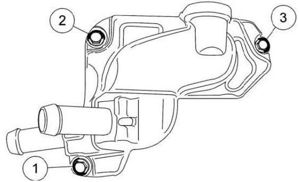
41. Install the 2 nuts for the fuel cooler.
