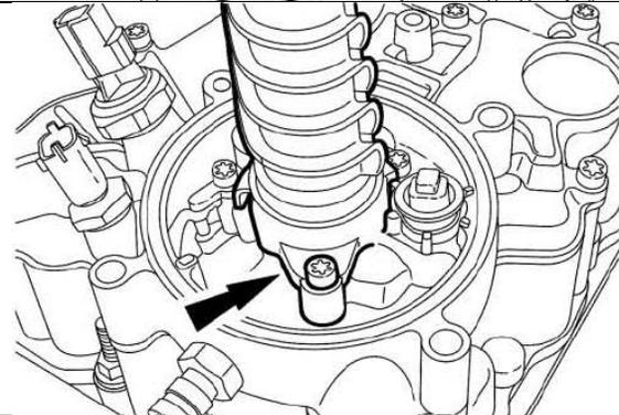
9. Install the oil filter housing and 4 Torx bolts.
