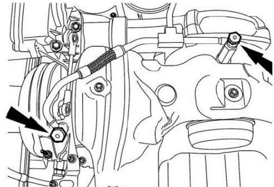
49. Position the auxiliary air intake (ACL) hose in the vehicle.
