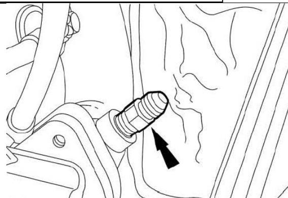
34. Connect the EP sensor tube to the EGR-OC pipe.
