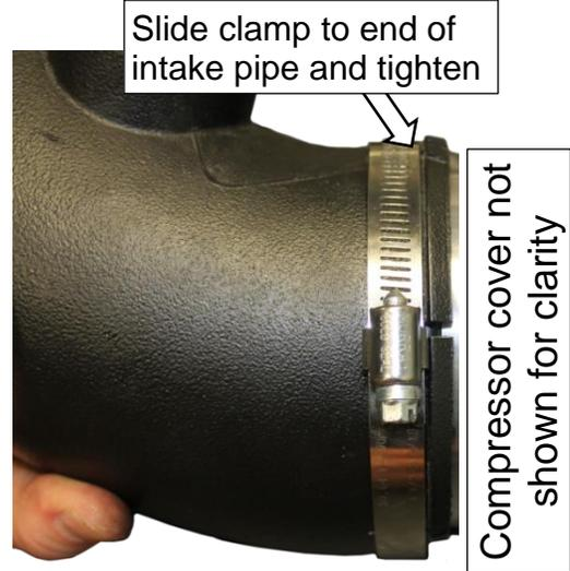
Slide clamp to end of intake pipe and tighten
