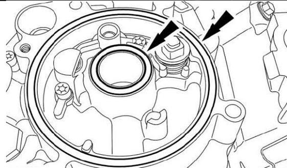
8. Install the oil filter return tube assembly and screw.
