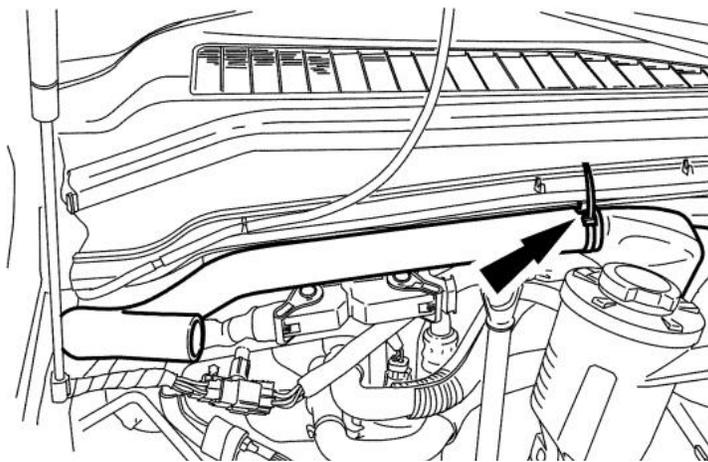
**1047082/83 ONLY** – Use supplied silicone boot and hose clamps to adapt the AFE intake to the BD Screamer turbo.
