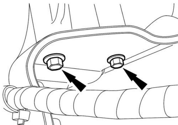
33. Remove the bolt for the engine wiring harness.
