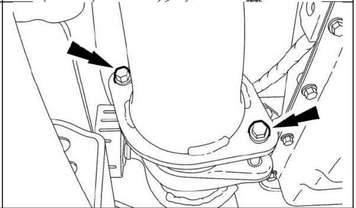
27. **NOTICE:** Failure to install and correctly tighten the Exhaust Gas Recirculation (EGR)-Oxidation Catalytic Converter (OC) pipe support bolts will result in damage to the horizontal EGR cooler and possible engine damage. Install the bracket, washers and loosely install the 2 new bolts for the EGR-OC pipe bracket.
