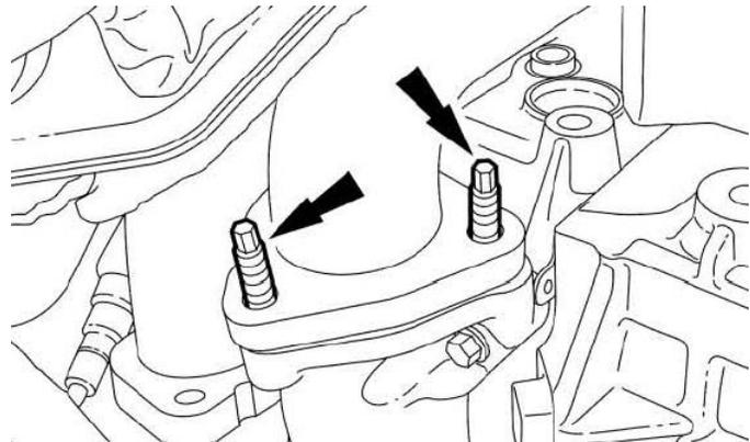
20. Install the new turbocharger inlet pipe gaskets, bracket and loosely install the 6 new bolts.
