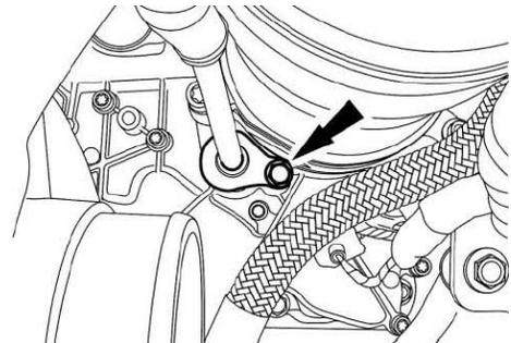
48. Prelubricate the oil inlet holes of the turbocharger assembly with clean engine oil and spin the compressor wheel several times to coat the bearings with oil.
