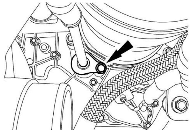
5. Remove the 5 bolts and the turbocharger heat shield.
