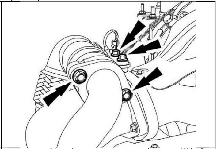
26. Tighten the 2 bolts for the exhaust downpipe at the OC.
