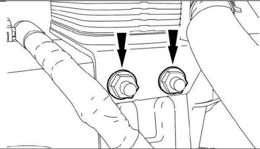
42. *NOTE:* It may be necessary to loosen the front bolts of the turbocharger crossover in order to get correct alignment of the holes for the fuel cooler.
