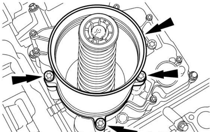
37. Remove the screw and the oil filter return tube assembly.
