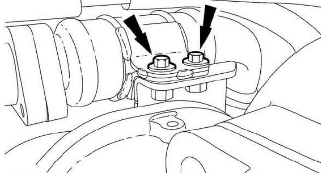
31. **NOTICE:** Failure to install and correctly tighten the Exhaust Gas Recirculation (EGR)-Oxidation Catalytic Converter (OC) pipe support bolt will result in damage to the horizontal EGR cooler and possible engine damage.
