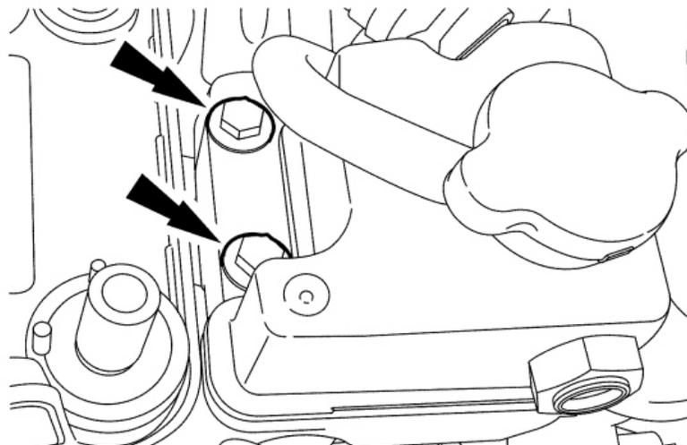
8. Remove the 2 bolts for the fuel cooler.
