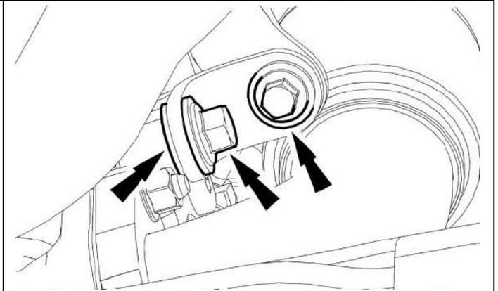
28. Install the new gasket and the 2 new bolts for the EOR-OC pipe at the EGR cooler.
