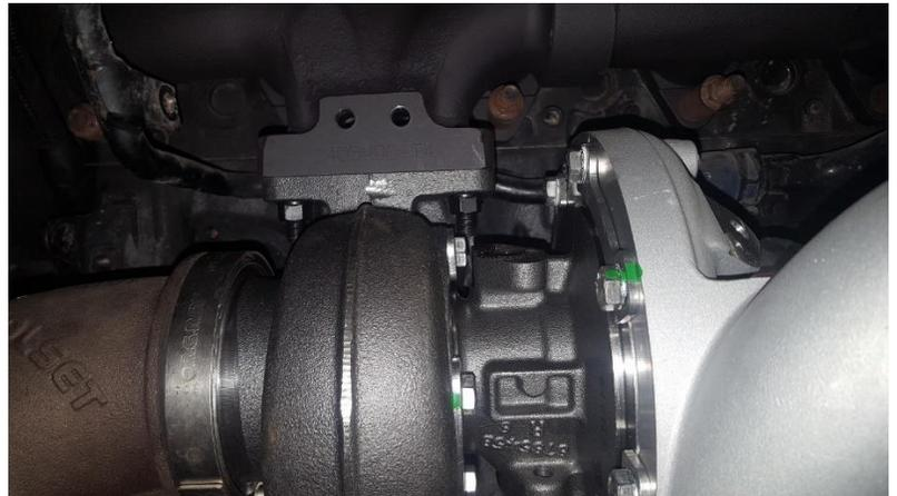
10. Check that there is approximately 1/4" clearance between turbo and shock tower. Clock turbo if required, see step 10.
