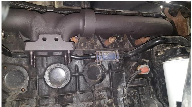
4. Install the coolant line bracket (1405998) as shown.
