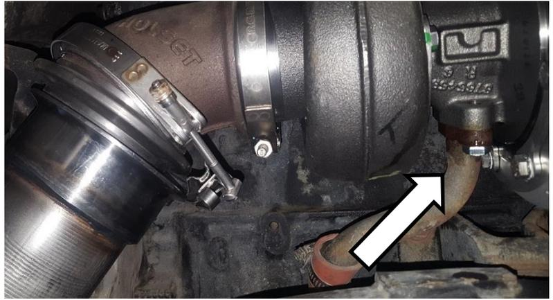
14. Install the oil supply line (reuse OE line).
