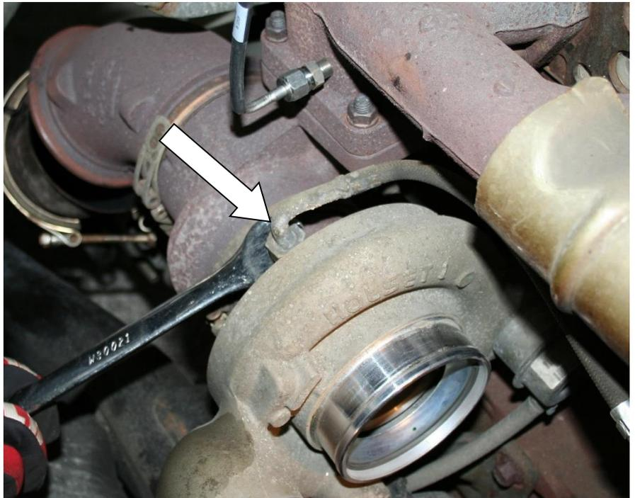
9. On 05-07 trucks, you will need to disconnect the wastegate solenoid connector.
