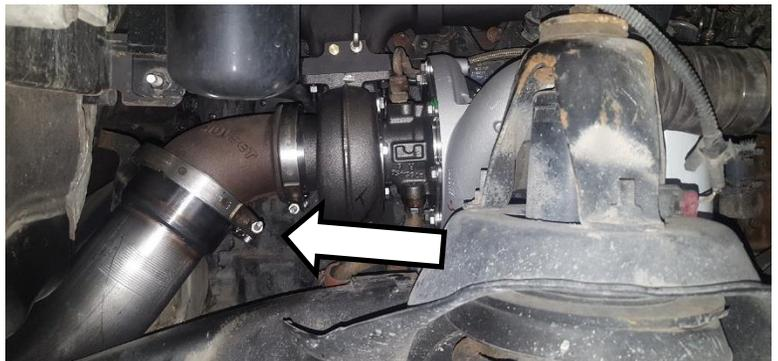
17. Install the intake tube and airbox.
