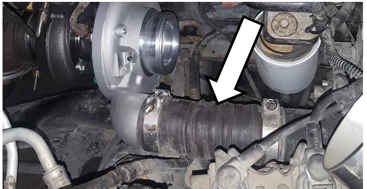
16. Connect the exhaust to the downpipe. Tighten clamp.
