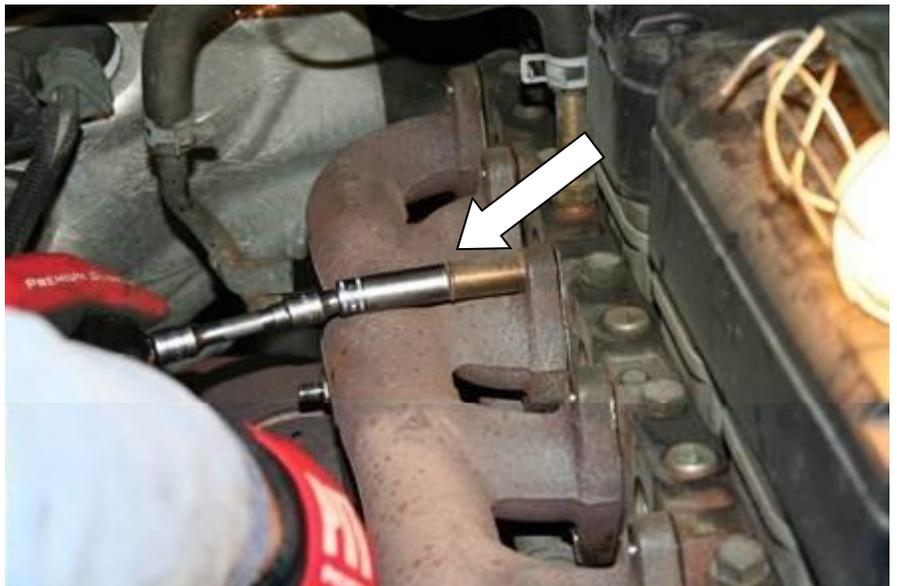
14. Remove the turbo/manifold assembly from the engine compartment.
