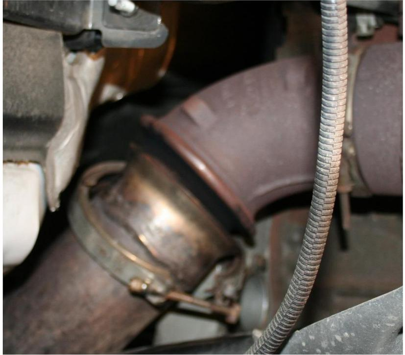
6. Remove the turbo oil drain line with a 10mm socket. Remove the oil drain out of the engine block.
