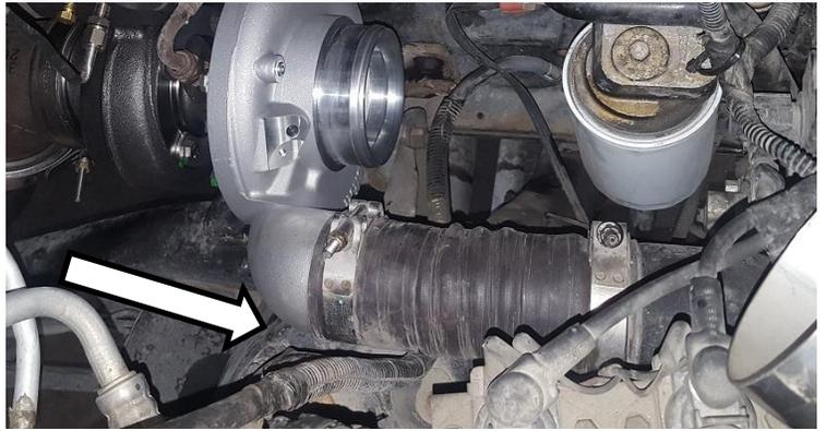
11. To clock turbo loosen all 8 bolts on turbo compressor housing and rotate the housing clockwise till there is approximately 1/4" gap between the housing and the shock tower.
