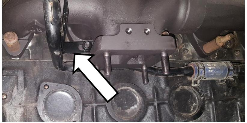
5. Drill a 5/16" hole on the cut off factory coolant bracket and use the provided hardware to secure the brackets together.
