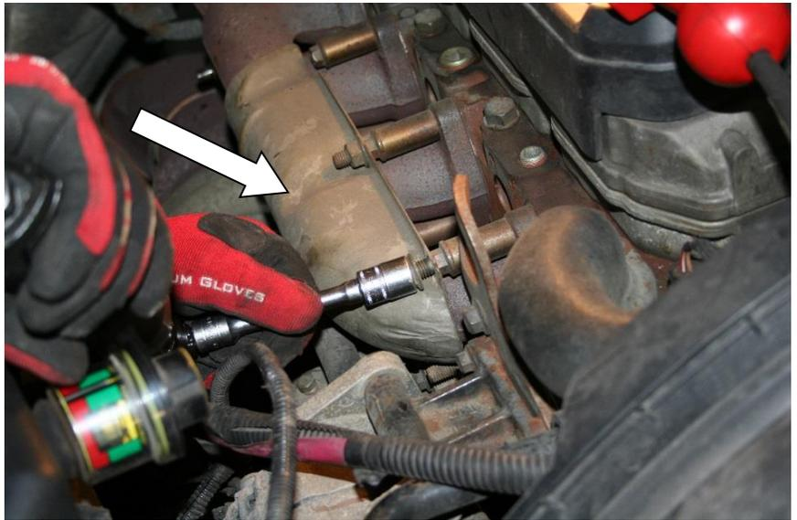
13. Remove the remaining manifold bolts using a 13mm socket.
