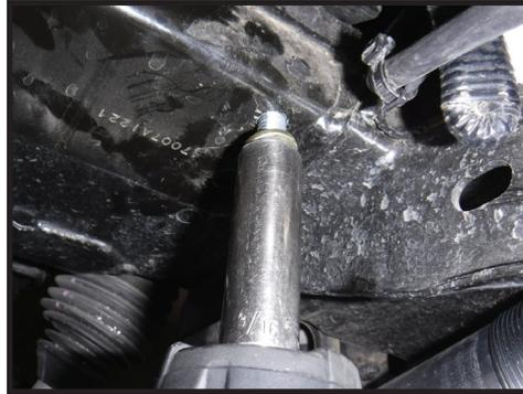
**13.** Mount the reservoir bracket using the self-tapping screw and a 9/16".
