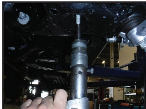
3. Remove the studs from the lower shock bar pin mount where it attaches to the lower arm. This can be difficult, it is recommended to use an air hammer to knock the studs out. It can be done with a heavy hammer or hand sledge. [FIGURE 2]
