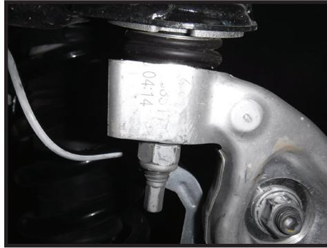
**5.** Separate the UCA from the spindle and support the spindle so that it does not overextend the CV joints when detached.
