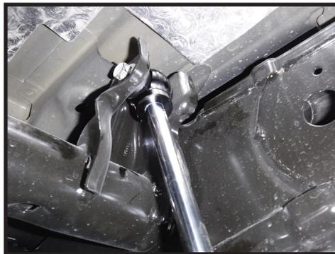
**4.** Mount the shock in the lower mount with the reservoir facing away from the axle. Make sure the nuts are properly retained in the sheet-metal retainers. Torque bolts to factory spec using a 15mm. [FIGURE 2]
