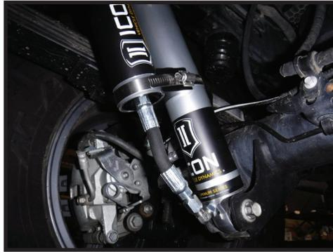
**5.** Install the ICON shock in the lower mount. Firmly press upward on the shock to compress it enough to line it up with the lower mounting hole and start the bolt. Make sure the nuts are properly retained in the sheet metal retainers. When tightening the lower shock bolt push up on the shock as much as possible to prevent contact with the mounting tabs, slight sanding of the mounting tabs may be necessary. Torque upper and lower shock bolts to factory spec using a 15mm. [FIGURE 3]
