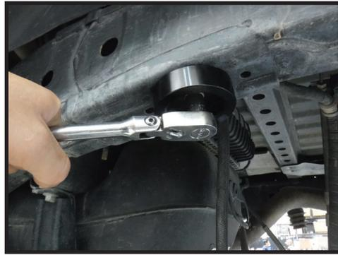
4. Snap the bump stop into the bump cup as shown. [FIGURE 5]
