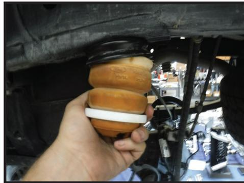
2. Using appropriate tools, remove the factory BUMP STOP cup by removing the center bolt.
