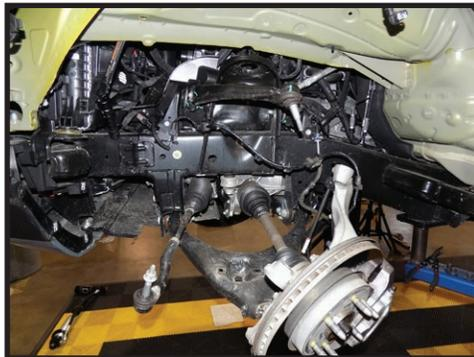
**11.** Grab the new ICON coilover and make sure the lower bar pin is oriented correctly for ease of bolt installation. This may require using an adjustable wrench or vise to rotate the barpin/bearing as shown. [FIGURE 12]
