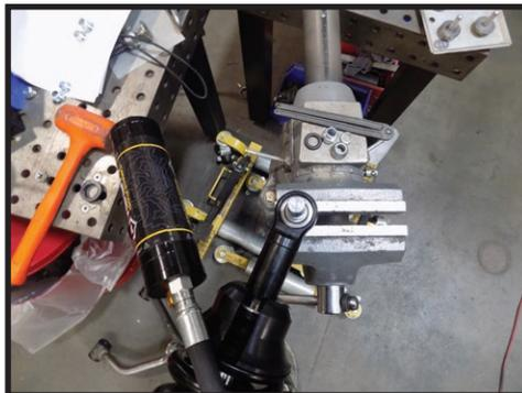
**12.** With the new ICON UCA installed into the frame mounts, place the ICON coilover into the coil bucket and lower arm. Apply thread locker to the OEM barpin hardware and insert it through the arm and into the barpin, do this by hand so as to not cross thread the bolts. Torque to 45 ft-lbs.
