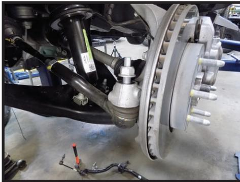
**6.** Next you will need to loosen and remove the upper joint nut using an 18mm. Then use the ball joint separator to break the ball joint taper free from the knuckle. A well-placed hit with a hammer onto the knuckle can also free the taper. Leave the nut attached so the knuckle does not fall away and pull apart the CV joints. [FIGURE 5]
