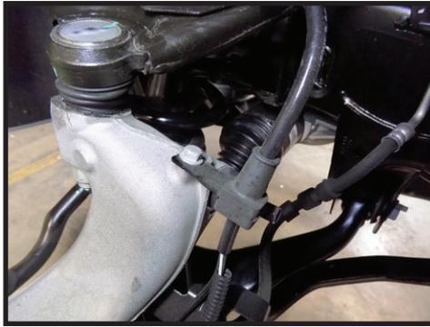
**5.** Remove the tie rod nut using a 21mm and remove the tie rod of the knuckle using a ball joint separator. [FIGURE 4]
