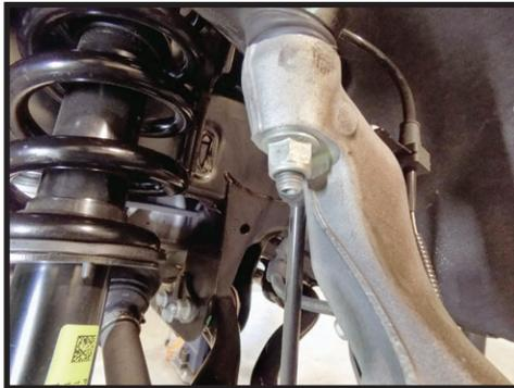
**7.** Now support the knuckle with a strap to the frame to keep it from falling away and pulling apart the CV axle. Then remove the nut from the upper ball joint. The knuckle should rotate out of the way to easier access the coilover.
