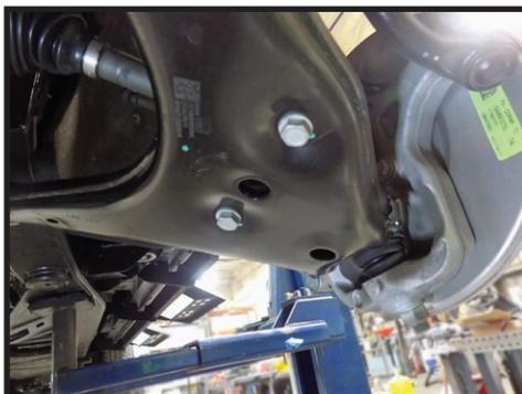
**9.** Remove the (3) 18mm nuts from the top of the coilover. There is a wire loom clip on one of the factory studs, use a screw driver or small pry bar to remove it (For easier access, half of the fender liner can be removed and folded out of the way using a T15 torx and plastic clip removal tool). [FIGURE 7-10]
