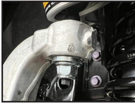
**13.** Install the ABS bracket onto the Billet UCA using the factory bolt. [FIGURE 15]
