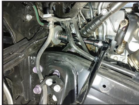
**7.** Locate the front driver side core support mount bushing. [FIGURE 7]
