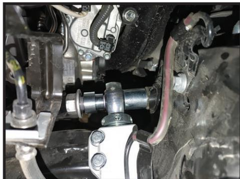
**12.** Install the Delta Joint Pro into the spindle, apply included blue thread locker to threads on flange nut and thread on to Delta Joint Pro with washer (605890) between the flange nut and spindle [Torque the nut to 70 ft-lbs]. [FIGURE 14]
