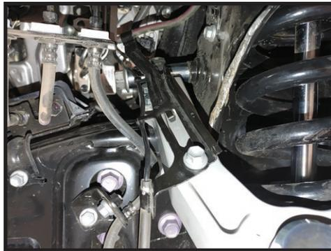
**14.** Torque the factory long pivot bolt to OEM spec.
