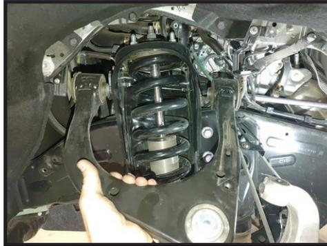
**10.** Prepare Icon Billet UCA for install. Be sure the heim spacers are correctly installed. Refer to photo. [FIGURE 11]
