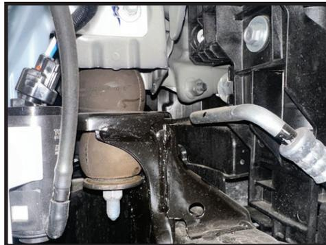
**8.** Using a jack carefully apply pressure to the driver front core support bolt this will lift the intercooler up enough to remove the UCA pivot bolt. [FIGURE 8 & 9]
