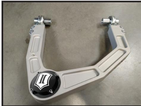
**11.** Install the ICON UCA into position and slide the factory mounting bolt through the heims, spacers and frame. [FIGURE 12 & 13]
