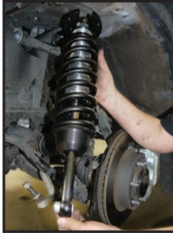
**8.** Connect the shock to the lower control arm: The lower shock mount has (1) long and (1) short spacer [Torque to factory spec]. Make sure the long spacer is toward the front of the vehicle as this will position the shock further toward the rear of the A-arm to ensure adequate sway bar clearance. Install the factory lower shock bolt.
