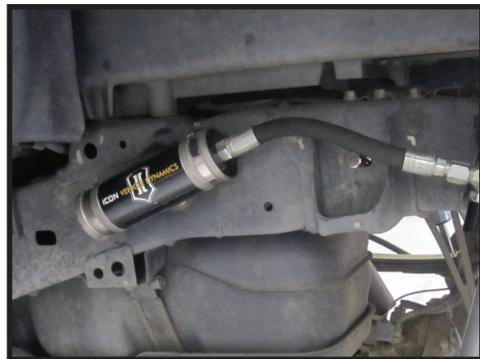
**11.** Thread the supplied (3/8" x 3/4") self tap bolt into the frame rail using a 9/16" socket/wrench, minimum of 2 full rotations.
