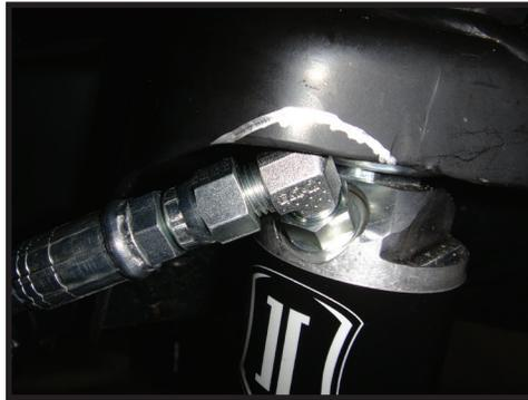
**7.** The hose must exit as pictured. [FIGURE 2] Allowing the reservoir hose to exit differently OR over tightening of the stem bushing lock nut will cause the reservoir fitting to collide into the frame. [FIGURE 3] Displays contact of the reservoir fitting and the frame when the shock is installed incorrectly.
