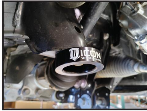
3. Install the poly bump stop into the cup. The small diameter side will slip into the cup. Start with one side and work your way around, keeping pressure applied until the poly bump snaps into place. [FIGURE 4]
