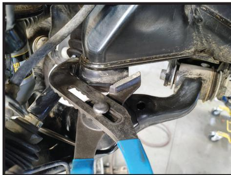
2. Take the ICON bump stop cup and 10mm bolt. Apply thread locker to the bolt threads. Install bump stop cup and bolt as shown. Torque to 30 ft-lbs. [FIGURE 2 & 3]
