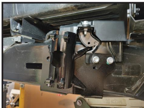
**22.** Using the bump stop bracket as a guide, drill the rear hole out to 1/2".
