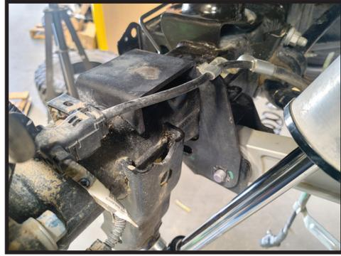
**4.** Install the supplied 1/2-13 x 1.000 grade 8 bolt, washer, black zinc washer into the link pocket thru the striker pad. Install second flat washer and nylock nut. Torque to 70 ft-lbs. [FIGURE 5, 6, 7]
