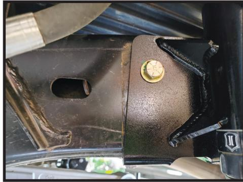
**13.** Insert the ICON 2.0 hydraulic bump stop into the mount and secure with the supplied 1/4-20 x 2.00 grade 8 bolts and nylock nuts. Torque to 8-10 ft-lbs. [FIGURE 16]
