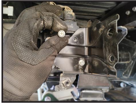
**17.** Remove the factory bumpstop using a 12mm. The bolts will be reused.
