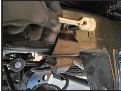
**9.** Remove the plastic caps from either side of the bump stop. Use a screwdriver to press in the clips and pry them out. [FIGURE 10 & 11]
