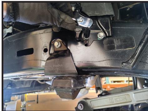
**15.** Remove the plastic cover from the fuel pump controller using a 12mm. [FIGURE 18]
