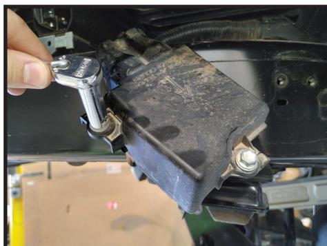
**16.** Remove the controller from the bracket and secure the controller so it does not stress the wiring. A #2 phillips or 8mm can be used to remove the 2 screws. [FIGURE 19]
