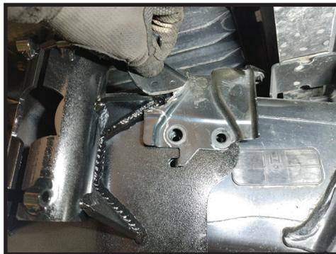
**21.** Reinstall the controller and plastic cover onto the bracket and install the bracket onto the frame, over the ICON bracket using the remaining 2 long bolts (1 from passenger side and 1 from driver side). Torque to 20 ft-lbs. [FIGURE 22]
