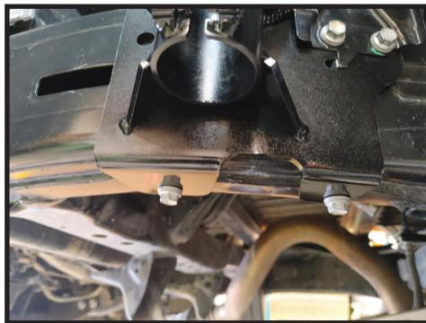
**20.** Take the fuel pump controller bracket and place it over the mounting holes and mark it to be cut to clear the bump stop bracket gusset. Cut it with a cut off wheel. Paint the exposed metal to prevent rust from forming. [FIGURE 21]
