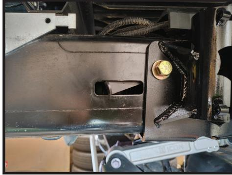
**24.** Slip the remaining hydraulic bump stop into the can and secure it with the 1/4-20 x 2.0 grade 8 bolts and nylock nuts. Torque bolts to 8-10 ft-lbs. [FIGURE 24]
