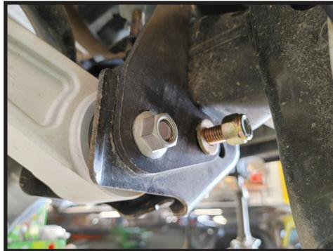
**5.** Torque the lower link bolt to factory specs. Hold the nut stationary with a 19mm while tightening the bolt. The nut can be damaged if rotated.
