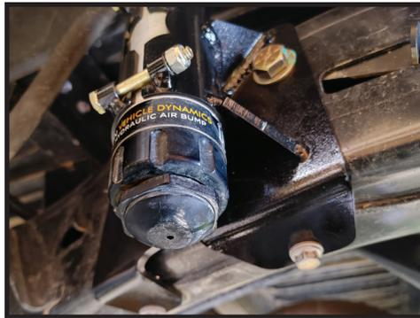
**11.** Use a 1/2" drill bit to drill out the holes thru the bump stop bracket into the frame. [FIGURE 13]
