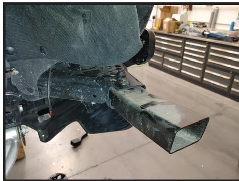
**7.** Install the new Icon crash bar into place, the ribs should face the tire and the kick should be up. Install the factory hardware using a small amount of vibratite red thread locker and torque to factory specs. **[FIGURE 6]**
