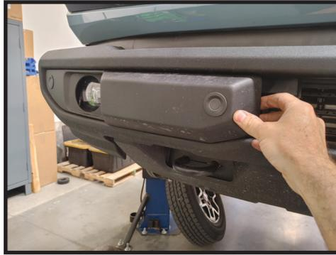
**5.** Using a 15mm, loosen the 3 bolts holding the bumper to the frame. **[FIGURE 4]**
