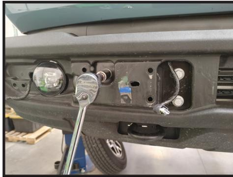
**6.** Using a 15mm loosen and remove the 2 bolts holding the front crash bar in and remove the crash bar. **[FIGURE 5]**
